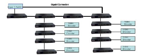
Figure 4: A multicast traffic through a 6K32T Switches with Gigabit redundancy
